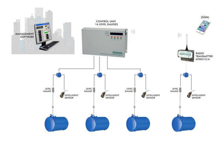
Level measurement and leakage alarm monitoring control unit for tanks, piping and wells. Management of 16 level guages and 16 leakage alarm sensors, 16 on/off inputs and up to 8 relays with programmable-event outputs. It can be connected to 4 other devices to extend the level, alarm and relay control and to allow interfacing with main control systems installed on refuelling stations.
